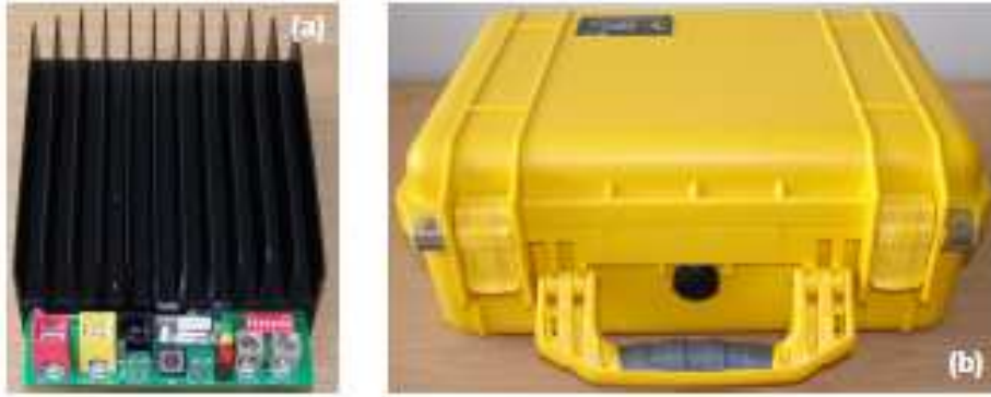
Figure 1.2 – a) TriStar 45 solar charge controller and b) 1450 PeliCase box.
